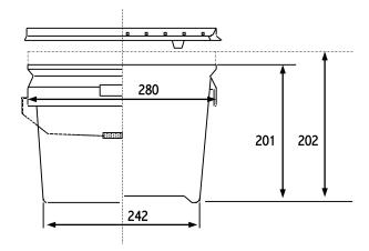
Measurements in millimetres
